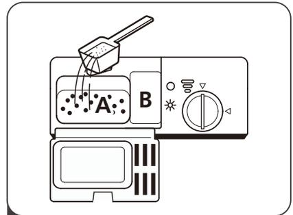
**2** Add detergent into the larger cavity (A) for the main wash. For more heavily soiled wash loads, also add some detergent into the smaller cavity (B) for **release during** pre-wash.
