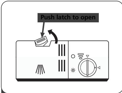
1 Press the release latch on the detergent dispenser to open the cover.
