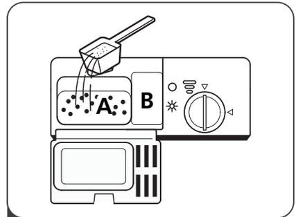
2 Add detergent into the larger cavity (A) for main wash. For more heavily soiled wash loads, also add some detergent into the smaller cavity (B) for release during pre-wash.
