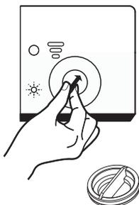
Remove the rinse aid reservoir cap. Turn the rinse aid indicator dial to a number. The higher the number, the more rinse aid the dishwasher uses.
